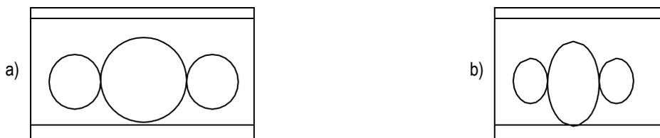
**Figure 2: Wide-screen film converted into HD 16:9 format (a) and SD 16:9 anamorphic format (b)**
